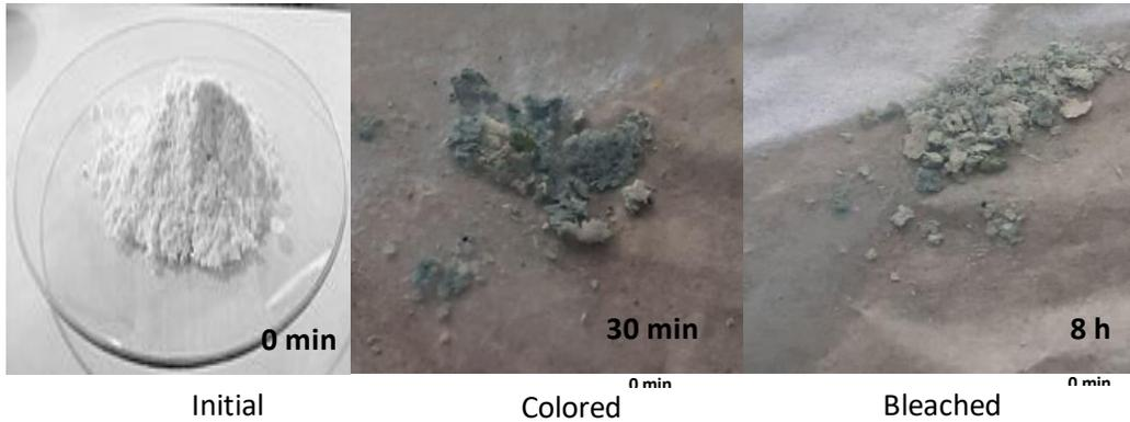
Figure 1. Show the color difference before UV and after UV irradiation and bleached state
