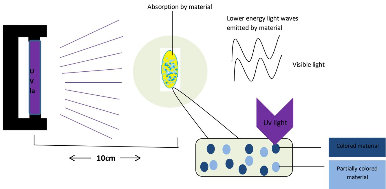
Scheme 2: Experimental setup of photochromic property of powder sample
