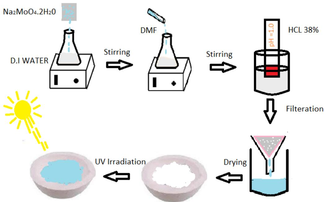
Scheme 1 :Schematic representation of step wise synthesis process of MoO<sub>3</sub> nano powder and photochromic property
